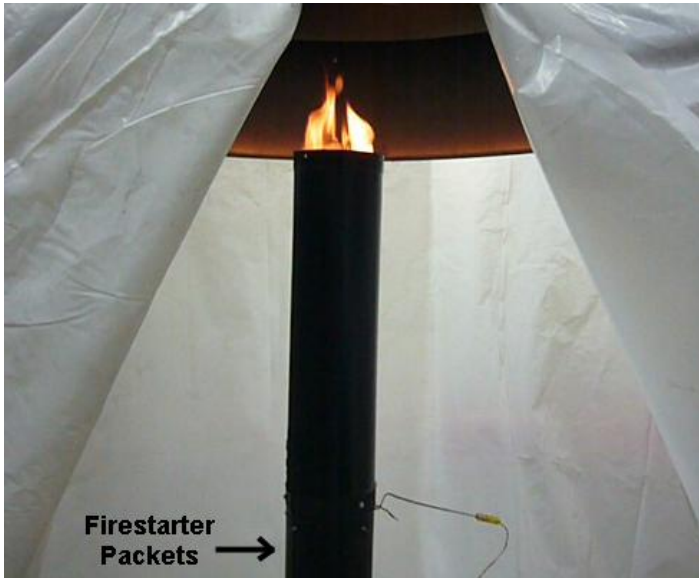
Figure 2. Simulated chimney fire, run 2
